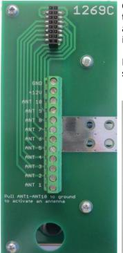
On the picture to the right the 12-position socket are shown where the control cable are connected. + 12V are common and each antenna is controlled by grounding resp. input at the socket. There is a extra ground connection also marked GND.
