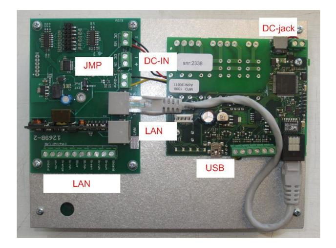
To reach the different connectors the top cover have to be removed. The top cover is secured to the bottom by 8 stainless steel M3 screws.
