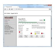
The RC-1216 can be configured to remote control a Expert 1K-FA Power amplifier. The daily used controls and indicators are available direct from the web interface. The RC-1216H also act as a serialport server so you can connect with the original PC-program in parallel if you have to do some setups.
