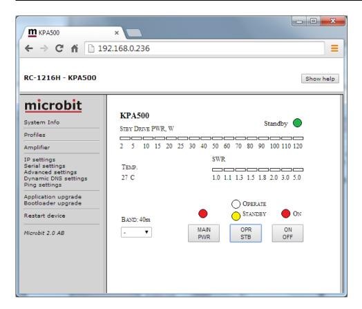
In standby mode the PWR scale will be rescaled to show the driving power from the TX.
