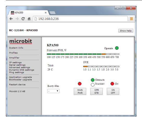
In operate mode the PWR scale is rescaled and are showing PA output power.
