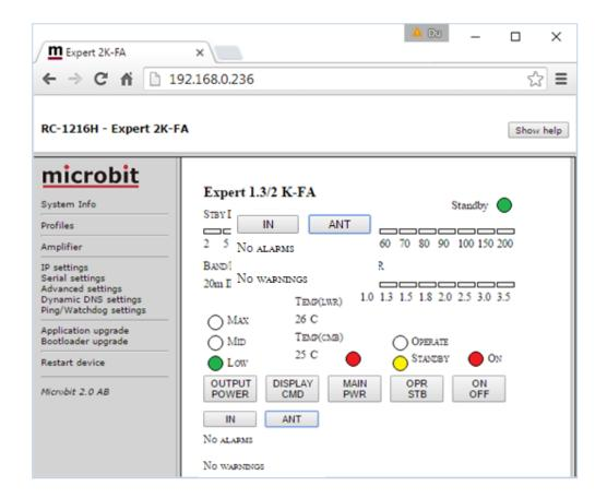
In standby mode the PWR scale will be rescaled to show the drive power from the TX.
