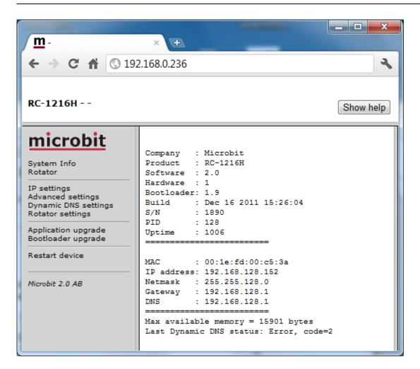
The info page shows some static information about the RC-1216H as firmware revision etc. and also the basic IP-configuration.
