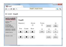
The RC-1216 can be configured to remote control a SteppIR antenna. The controls are the same as on the SDA-100 control box. You can use Retract, Calibrate, Bi-directional, 180 degree switch etc. Frequency adjustment can be done manual or automatic.
