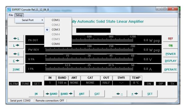
When you have selected serial port go back to the Setup Manager Window and click on the refresh button. Now Port status should change to "Connected".
