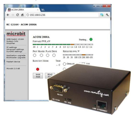
The RC-1216 can be configured to remote control a ACOM-2000A Power amplifier. The controls and indicators are almost the same as on ACOM-2000A control Panel (RCU) so you will recognize them immediately. There are controls for on/off, standby/operate, Auto tune, Antenna selections and a button for reading all parameters from the PA. The indicators are also the same as on the RCU like Forward power, Reflected power, Alarm LED:s, Band segment, Temp indicators etc.
