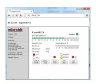
The RC-1216 can be configured to remote control a Expert 1.3K-FA Power amplifier. The daily used controls and indicators are available direct from the web interface. The RC-1216H also act as a serialport server so you can connect with the original PC-program in parallel if you have to do some setups.
