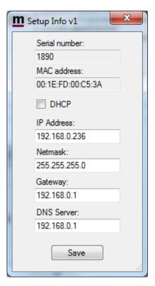
A new window wills pop-up with the basic IP settings. Change the settings so they fit into your local network and press the "Save" button to save the new settings. The RC will restart again and when the text "1216H-connected" shows up again in the lower field of the Setup-Manager, you can click on the "Setup" button again to verify the changes.
