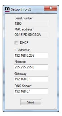
(\*) In most cases the Gateway and the DNS server is the same and the IP of the router.
