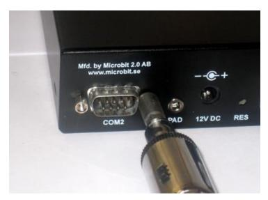
2: Open the box by pressing the D-sub until you can get your fingers behind the edge of the lid and can slide the housing apart.
