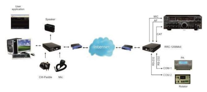
RRC-1258MkII supports the YAESU CAT protocol used by almost every YAESU radio. Then you have to use a PC-software e.g. HamRadioDeLuxe or similar rig control software at the control site. All audio and data communication goes true the RRC:s and you don't need a PC at the remote site.
