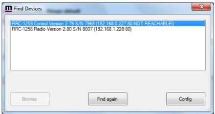
The RRC will reboot, when it's rebooted the "Find Devices" window will show the new IP (in this example 192.168.1.228) and the "NOT REACHABLE" text will not be shown.
