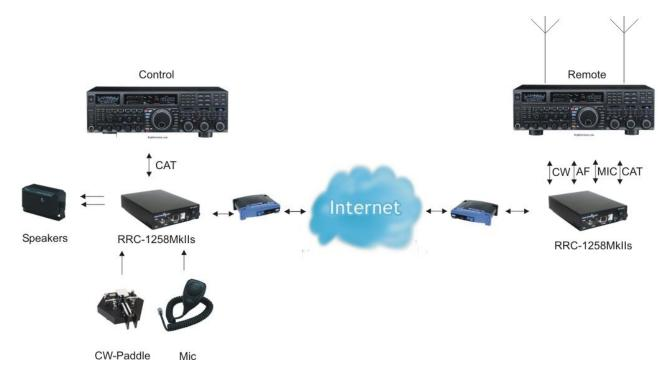
RRC-1258MkIIs Yaesu Twin supports the special high end concept where one Yaesu radio can be used to control another Yaesu radio. No PC:s needed at either end. The RRC-1258MkIIs Yaesu Twin package includes power supplys and all necessary cables. The boxes do not need to be opened all strappings are done in production. All you need to do is to put the system together and do the IP-settings.
