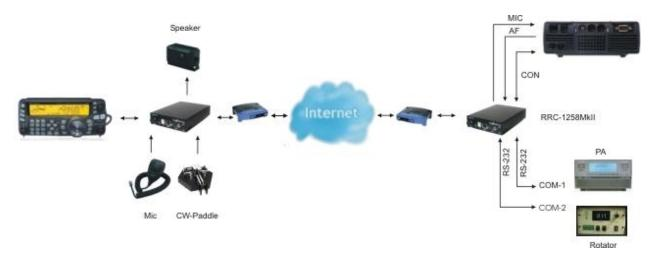
You will get the ultimate function of the Remoterig system together with radio stations with detachable control panels like Elecraft K3/0-mini-K3/100, Kenwood TS-480, Kenwood TM-D710, Kenwood TS-2000, Yaesu FT-857, ICOM IC-7100, IC-703, ICOM IC-706, IC-2820 and Alinco DX-SR8. You simply replace the cable between the control panel and the radio with the Remoterig system. You will get the same feeling and functionality as with the original setup.
