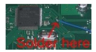
There is one solder pad which is significantly bigger than the other via holes to the right of the CPU over the Crystal. That's the one which the cables should be soldered to.
