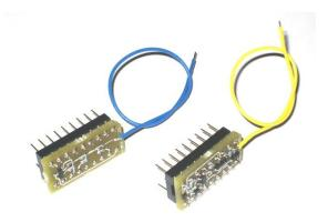
The small pcbs are mounted in the strapping sockets which means that no red straps are needed. The pcb with the yellow cable are mounted in the Control-RRC and the pcb with the blue cable are mounted in the Radio-RRC. The yellow and blue cables need to be solder to one point on the RRC pcb. See pictures below. Be sure to remove power when solder. There No settings need to be changed after mounting the pcbs.
