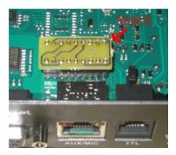
For your reference the picture below shows how the strappings are done on the small pcb.
