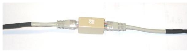
When you have finished both cables , you can connect them together with a RJ45 extender.
