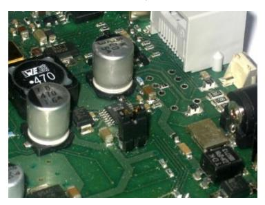
6: JMP-3 is placed next to the rear D-sub COM2. JMP-3 is used to connect RTS and CTS together (pin 7 and 8) in COM2. Most of the Yaesu and Kenwood radios with RS-232 port need to have them tied together. This is convenient if you want to use a prefabricated fully connected cable.
