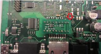
The picture below shows the configuration of the Radio-RRC:s. Note that the picture showing the Control side red straps are only valid for the first version of the IC-7100
