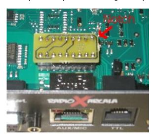
For your reference the picture below shows how the strappings are done on the small pcb.
