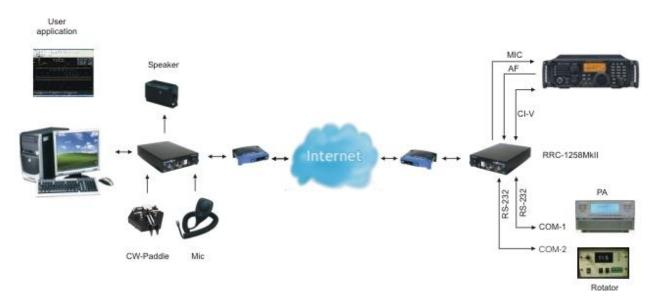
RRC-1258MkII supports the CI-V protocol used by almost every ICOM radio. Then you have to use a PC-software e.g. HamRadioDeLuxe or similar rig control software at the control site. All audio and data communication goes true the RRC:s and you don't need a PC at the remote site. The Connect/Disconnect button on the web status page is used to connect/disconnect to/from the remote site. It can also be done by the UP-button on the microphone or be set to always be connected.
