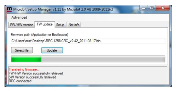
After about a 1 minute the update is finished and the RRC will restart. When the text "RRC-connected" shows up again in the lower field of the Microbit Setup Manager, you can change to the "FW/HW" tab and check software version.
