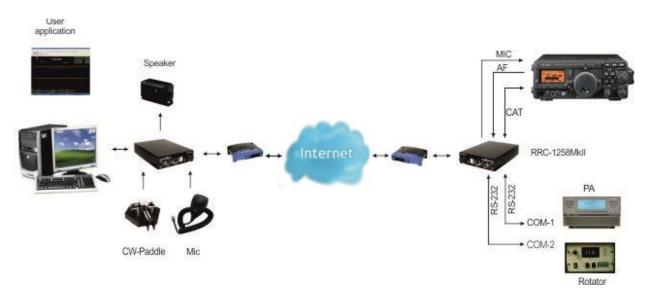
RRC-1258MkII supports the YAESU CAT protocol used by almost every YAESU radio. Then you have to use a PC-software e.g. HamRadioDeLuxe or similar rig control software at the control site. All audio and data communication goes true the RRC:s and you don't need a PC at the remote site.
