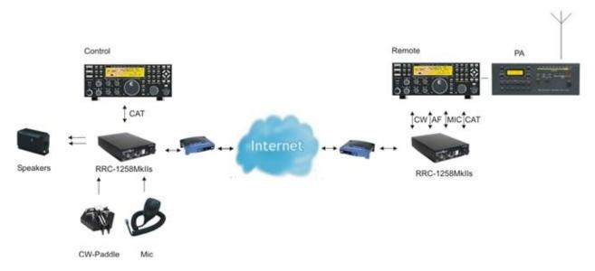
The twin solution for Elecraft K3 and Yaesus is the high end solution for the DX-er or contester who do not want to compromise in the selection of radio. The Twin solution is based on the idea that one local radio controls the remote radio and you get the feeling that you have the radio at your control site. For the Elecraft K3-Twin solution there is also a special K3 called K3/0-mini available which is specially designed to use as control as it has no RF-parts.
