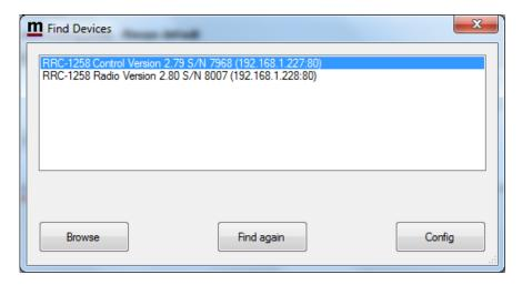
After the RRC has rebooted, the "Find Devices" window will show the new IP (in this example 192.168.1.227) and the "NOT REACHABLE" text will not be shown.
