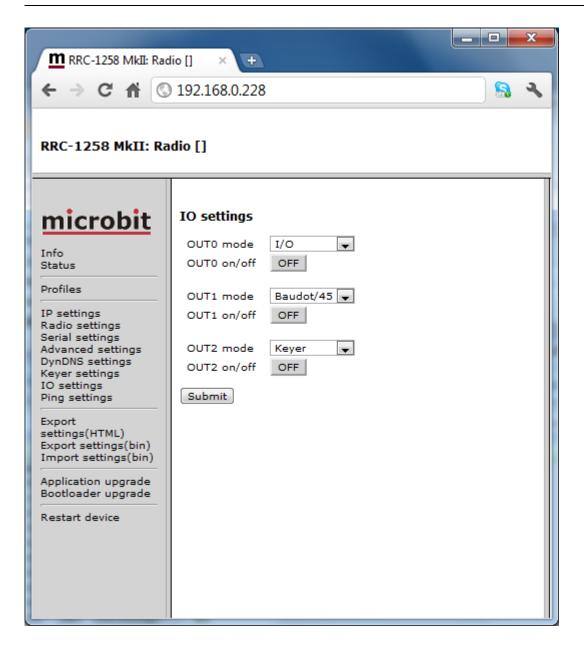
At the Radio-RRC IO-settings page you need to select which output you want to use for the RTTY keying signal. RTS from the RRC-1258 COMExtra USB port is used to key PTT.
