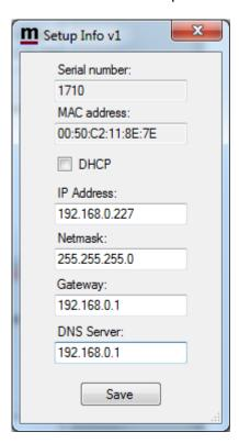
A new window wills pop-up with the basic IP settings. Change the settings so they fit into your local network and press the "Save" button to save the new settings. The RRC will restart again and when the text "RRC-connected" shows up again in the lower field of the Setup Manager, you can click on the "Setup" button again to verify the changes.
