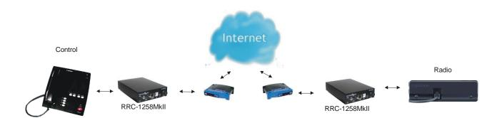
The RRC versions with 2-wire and 4-wire interfaces are mainly used for remote control of commercial radio systems which was designed for leased 2 or 4 wire lines. The interfaces are balanced and are using transformers for isolation nominal impedance is 600 ohm resistive. The 4-wire version can be order with opto couplers for transfer of E and M signals. Nominal audio level is -10 dBm and max level is about +4 dBm. The system also supports transfer of two independent serial ports.
