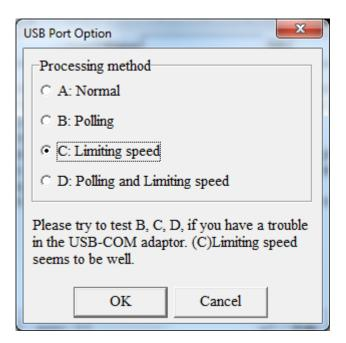
In the "USB port option" dialog select "C-limiting speed". If not limiting speed is selected the PTT will be released before the whole RTTY string is sent, because the USB communication is so much faster than a ordinary RS-232 serial port.
