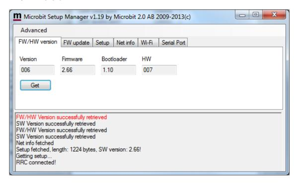
When you connect the RRC the version of the firmware and Bootloader will show up in the upper window. The hardware versions is also shown. Go to the page <a href="www.remoterig.com">www.remoterig.com</a> and under downloads you can find the latest firmware. If there is a newer firmware available download it to your desktop unzip it and change to the "FW-update" tab.
