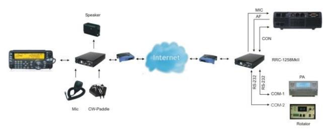
The idea of remote controlling TS-480 is simple; it's just to extend the cord between the radio and the control panel using Internet. When you press the power button on the panel the radio comes to life at the remote side and sound and panel info flows across the Internet between the pair of RRC-1258MkII:s. The look and feel of the panel is the same as if the panel was directly connected to the radio.
