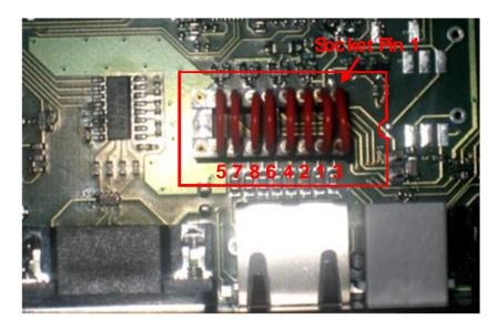
4: Control-RRC only: JMP-1 is placed behind the TTL connector. With the strap in place a DC voltage is feed to the microphone element. All ICOM microphones should be DC-feed. Dynamic microphones like the ones used by Kenwood should not be DC-feed. HEIL microphones should not be DC-feed either.
