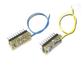
The small pcbs are mounted in the strapping sockets which means that no red straps are needed. The pcb with the yellow cable are mounted in the Control-RRC and the pcb with the blue cable are mounted in the Radio-RRC. The yellow and blue cables need to be solder to one point on the RRC pcb. See pictures below. Be sure to remove power when solder. There is no settings that need to be changed after mounting the pcbs.
