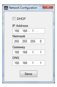
A "Network Configuration" dialog window will pop up. The Netmask, Gateway and DNS settings will be filled in already, they are copied from your PC:s Networks setting and normally do not need to be changed. The first 3 groups of the IP number are also filled in to match your PC-network settings.
