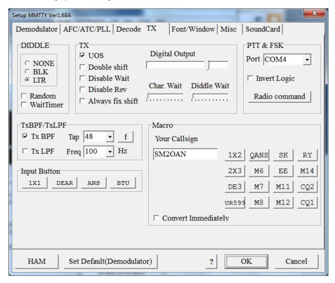
At the TX tab select the PTT & FSK comport to the same comport as Device Manager showed to be assigned to RRC-1258 COMExtra port, in this example it's COM4.
