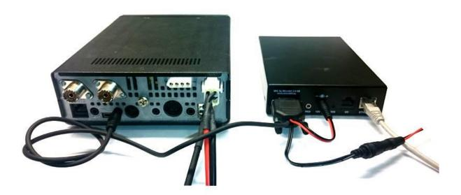
Set the radio CI-V baudrate to 9600 baud, this is done from the radio frontpanel. Setup the RRCs to match. If you only want to use RRC-Micro or RRC-Nano only the Radio-RRC settings are needed. You have to decide if you want to use the RS-232 or the USB connector for the connection to the PC (Yes = USB, No = RS-232)
