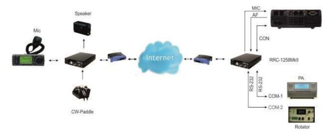
The idea of remote controlling IC-703/706 is simple; it's just to extend the cord between the radio and the control panel using Internet. When you press the power button on the panel the radio comes to life at the remote side and sound and panel info flows across the Internet between the pair of RRC-1258MkII:s. The look and feel of the panel is the same as if the panel was directly connected to the radio.
