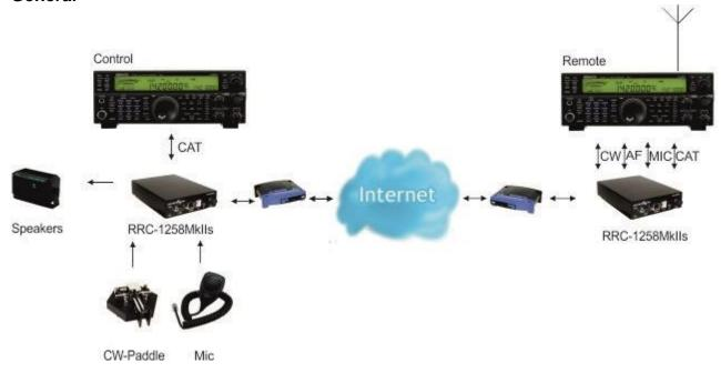
Finally we have implemented firmware for the Remoterig RRC-1258MkIIs to support Kenwood TS-590 in a twin setup like we have done for Elecraft and Yaesu before
