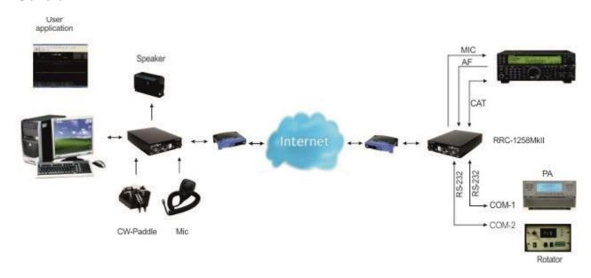
RRC-1258MkII supports the Kenwood protocol used by almost every Kenwood radio. Then you have to use a PC-software e.g. HamRadioDeLuxe or similar rig control software at the control site. All audio and data communication goes true the RRC:s and you don't need a PC at the remote site.
