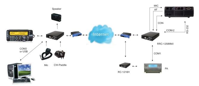
If you also need a connection for a PA or something which have to talk to the radio, it can be connected to Radio-RRC COM1 then the data will be mixed (under control) so both the PC and the PA can talk to the radio. Be aware of the pin configuration of COM1 it's not the same as for COM2
