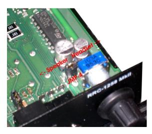
8: JMP-5 is placed behind the TLL connector and is only present in the RRC-1258MkIIs from hardware version 7. JMP-5 is used to decide if pin1 in the TTL connector should be grounded or not. It should be grounded (in place) for all Radios but Yaesu FT-857 and ICOM ID-E-880
