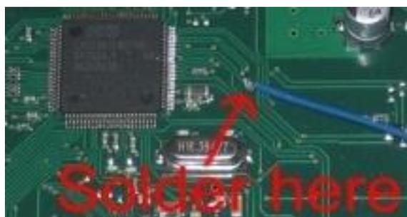
There is one solder pad which is significantly bigger than the other via holes to the right of the CPU over the Crystal. That's the one which the cables should be soldered to.
