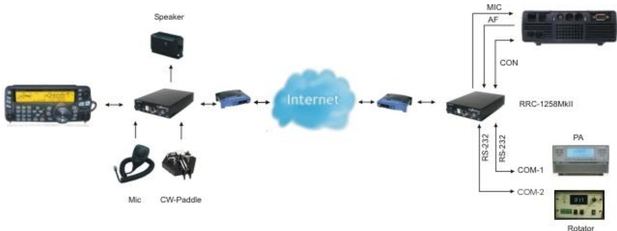
The idea of remote controlling TS-480 is simple; it's just to extend the cord between the radio and the control panel using Internet. When you press the power button on the panel the radio comes to life at the remote side and sound and panel info flows across the Internet between the pair of RRC-1258MkII:s. The look and feel of the panel is the same as if the panel was directly connected to the radio.
