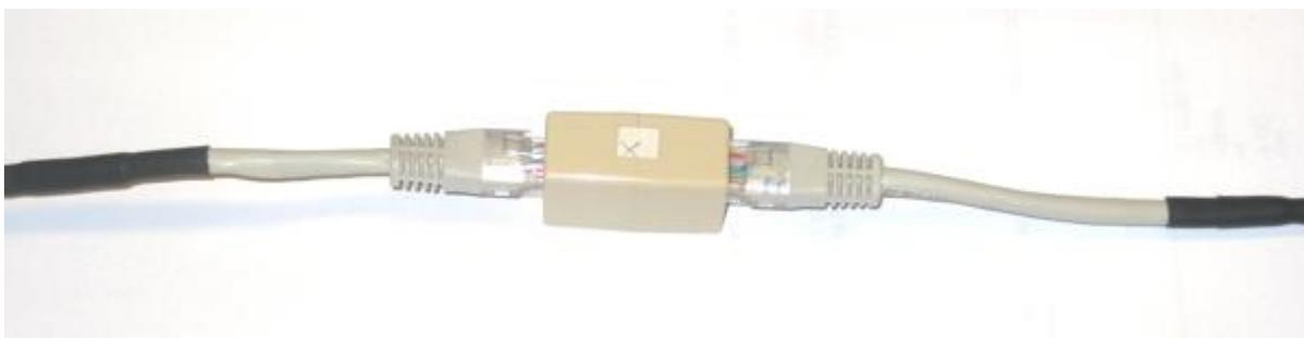
When you have finished both cables , you can connect them together with a RJ45 extender.
