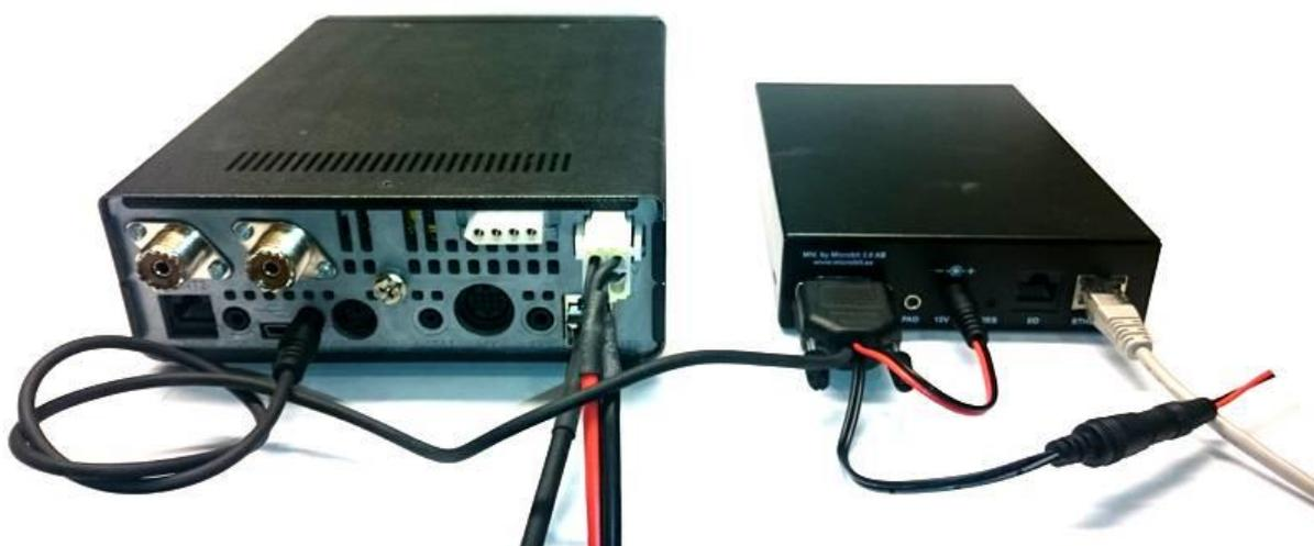
Set the radio CI-V baudrate to 9600 baud, this is done from the radio frontpanel. Setup the RRCs to match. If you only want to use RRC-Micro or RRC-Nano only the Radio-RRC settings are needed. You have to decide if you want to use the RS-232 or the USB connector for the connection to the PC (Yes = USB, No = RS-232)
